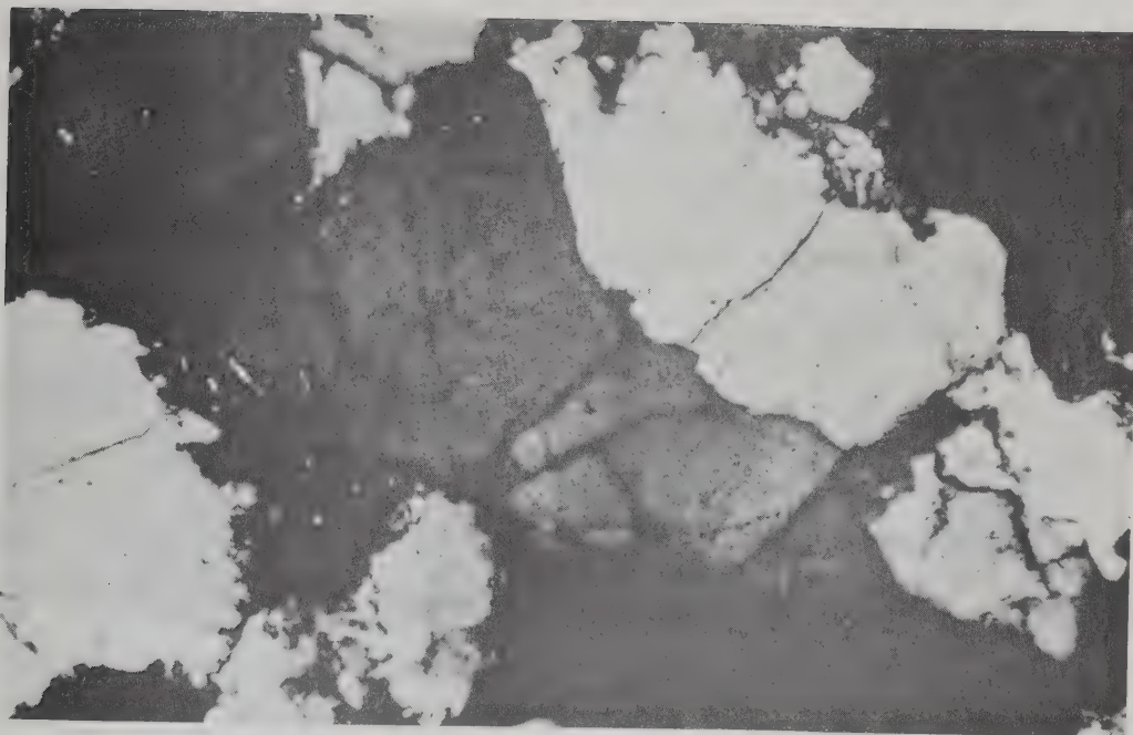
PLATE 7.7a Orthoquartzite from the Rocky Mountains showing extensive suturing at all grain contacts. Porosity is less than 5%. X130.
